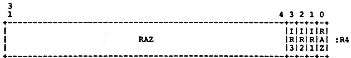
Figure 8-20: Software Interrupt Summary Register (SISR)
