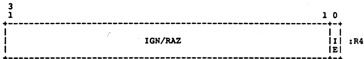
Figure 8-10: Interval Clock Interrupt Enable Register (ICIE)
