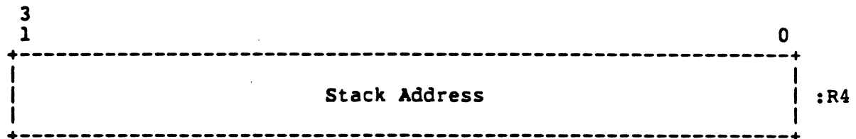
Figure 8-9: Stack Pointer Registers (ESP, SSP, USP)
