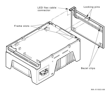
Figure 4–3 RZ56 Disk Drive Bezel Removal
