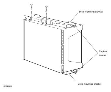
Figure 2-3 Installing Drive Mounting Brackets on an RZ56 **Drive for Any Slot Except the Rightmost Slot**
