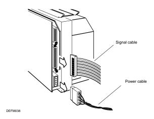
Figure 4-1 Disconnecting the RZ56 Disk Drive Connectors
