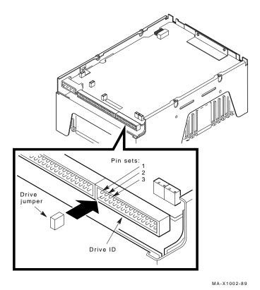
Figure 2-4 Setting RZ56 Disk Drive SCSI ID Jumpers
