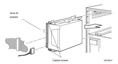
Figure 4–2 Removing an RZ56 Disk Drive
