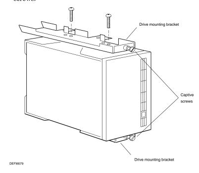
Figure 2–2 Installing Drive Mounting Brackets on an RZ56 Drive for the Rightmost Slot
