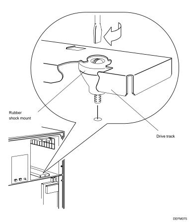
Figure 2–1 Installing the Drive Shock Mounts
