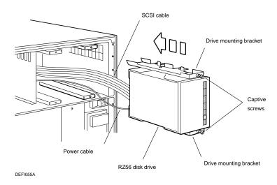
Figure 2–5 Installing the RZ56 Disk Drive in the Rightmost Slot
