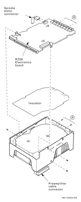
Figure 4-4 RZ56 Disk Drive Electronic Module Removal
