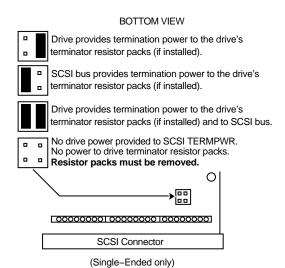
The following figure shows the proper placement of the terminator resistor packs on the RZ35/26 drive model.
