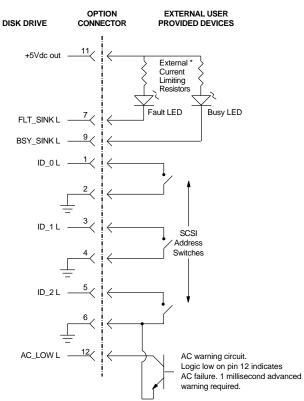
\* The 470 ohm current limiting resistors on the module are not shown in this drawing.
